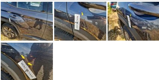
Door RR, Dent(s), Repair and paint (complete)
