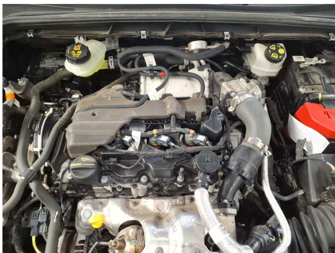
Missing part 1: Engine: Engine cover - Missing - Replace
