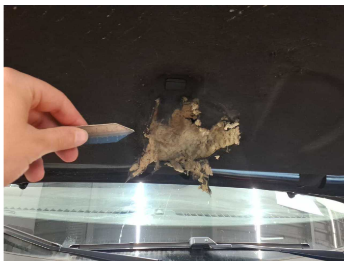
Damage 6: Bonnet: Insulation lining - Damage caused by marten / rodent - Replace
