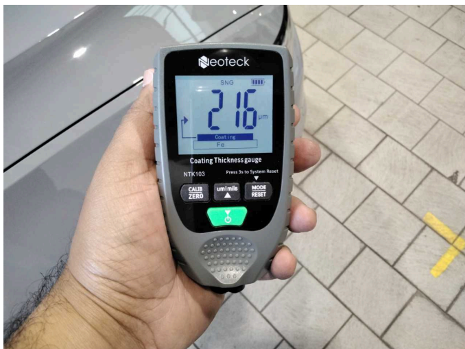
Mudguard - right side: 216 µm
