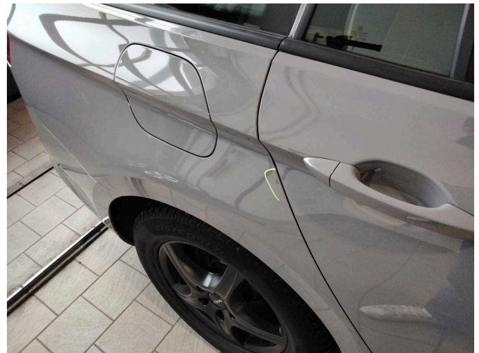
Wear and tear 5: Side panel - rear right side: Side panel - dent(s) - No deduction
