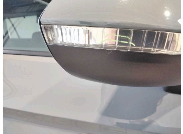
Wear and tear 3: Wing mirror - right side: Mirror housing - Scratch(es) - No deduction
