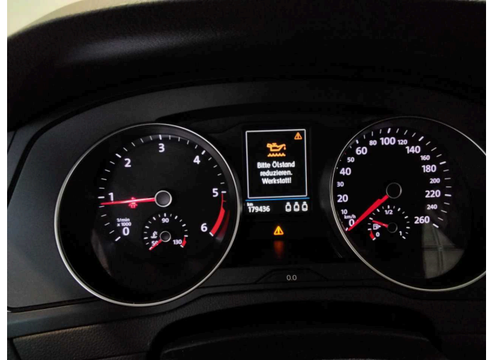
Damage 3: Instrument panel: Indicator light (Ölstand reduzieren) - on - Perform diagnosis
