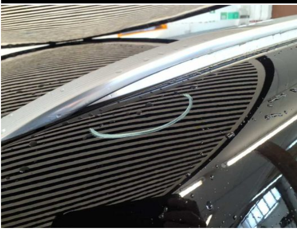
Damage #8: Body: Body (Mehrkosten möglich) - Damage by hail - Smooth repair work
