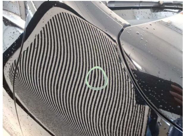
Damage #8: Body: Body (Mehrkosten möglich) - Damage by hail - Smooth repair work
