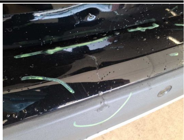
Damage #7: Rear bumper: Rear bumper - Deformed - Replace
