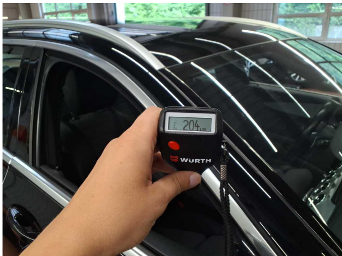
Repainting 1: Roof rail - right side
