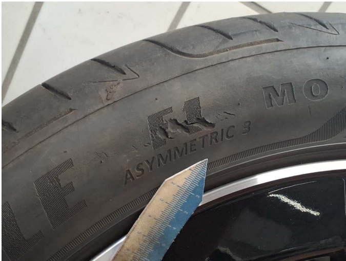
Damage 12: 2nd wheel set: 2 tyres - Broken / torn - Replace
