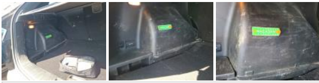
Internal boot lining R, Scratch(es), Replace
