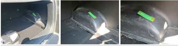
Rear bulkhead lining, Scratch(es), Smart repair
