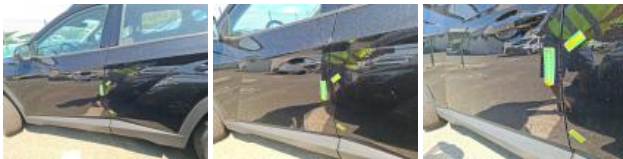
Door RL, Stone chip(s), Paint
