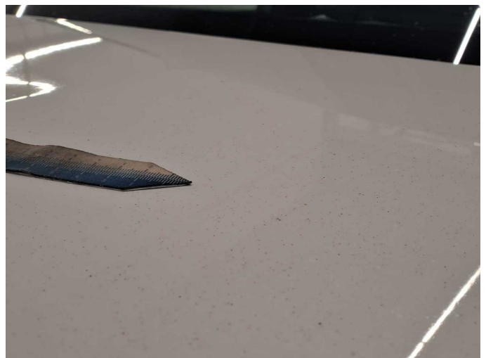
Damage 1: Body: Body (Flugrost) - Corrosion - Conditioning
