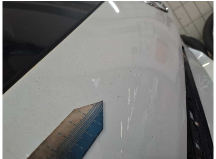
Damage 1: Body: Body (Flugrost) - Corrosion - Conditioning
