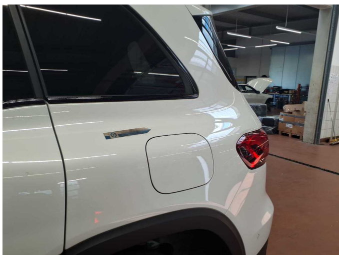
Damage 1: Body: Body (Flugrost) - Corrosion - Conditioning
