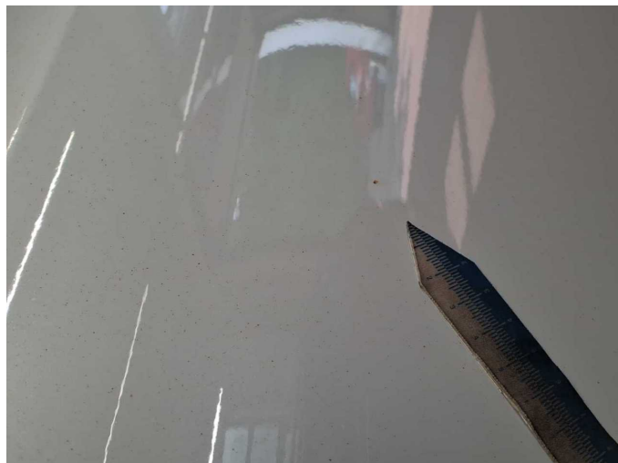
Damage 1: Body: Body (Flugrost) - Corrosion - Conditioning
