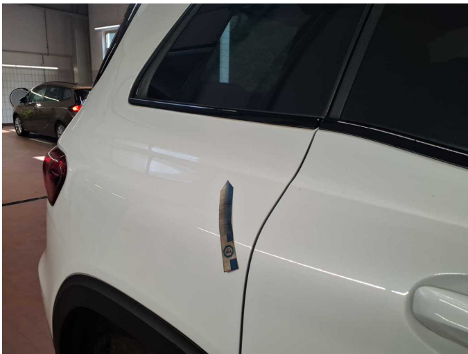
Damage 1: Body: Body (Flugrost) - Corrosion - Conditioning
