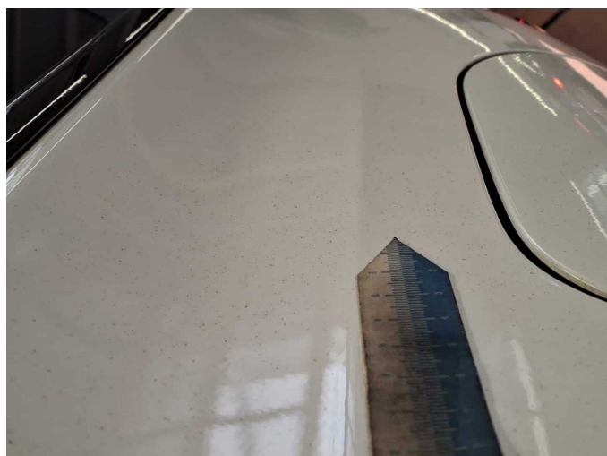
Damage 1: Body: Body (Flugrost) - Corrosion - Conditioning
