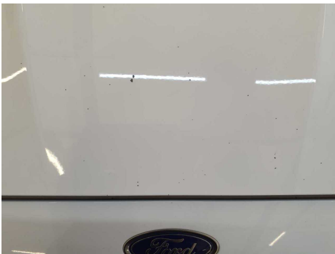
Damage 6: Bonnet: Bonnet - Stone chips - Paint
