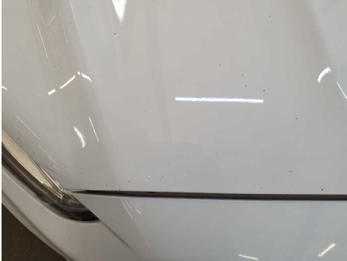
Damage 6: Bonnet: Bonnet - Stone chips - Paint
