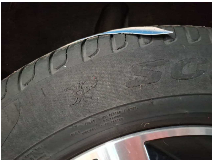
Damage 1: Wheel / tyres: Tyre - right - Broken / torn - Replace
