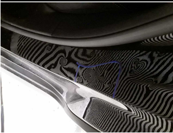
Damage #8: Side panel - rear left side: Sill - Dent / paintcoat damage - Repair and paint
