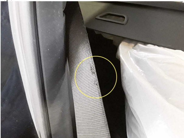
Damage #4: Seat belts - rear: Seat belt - rear right side - Porous / cracked - Replace
