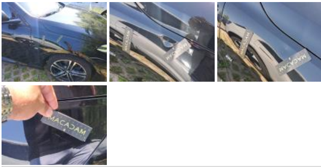
Outside rear-view mirror housing R, Scratch(es), Acceptable
