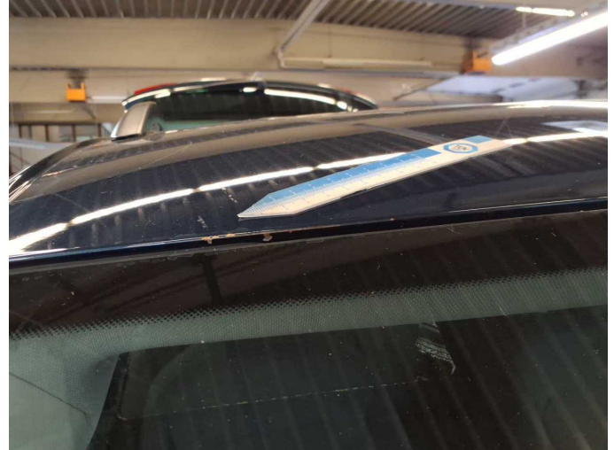
Damage 4: Roof: Roof - Corrosion - Paint
