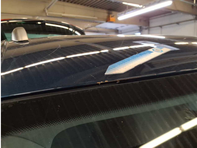
Damage 4: Roof: Roof - Corrosion - Paint
