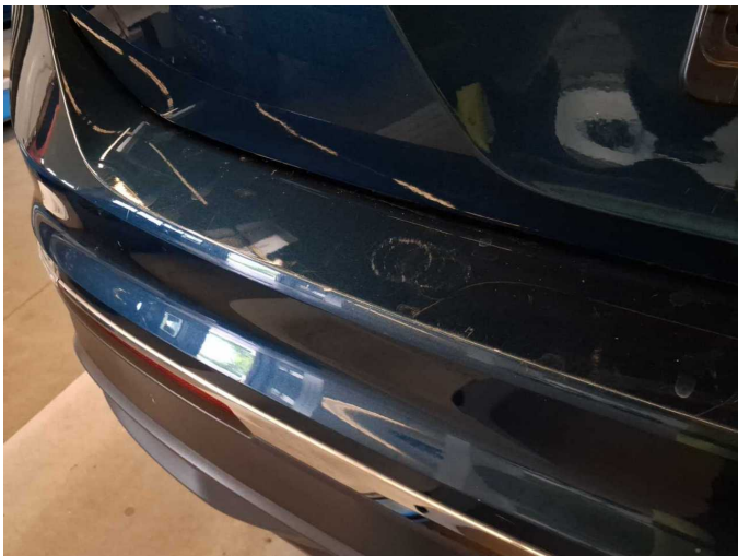
Damage 2: Rear bumper: Rear bumper (Ladekante) - Scratch(es) - Smart repair
