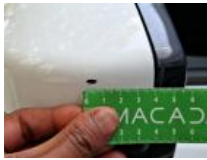
Outside rear-view mirror base L, Scratch(es), Repair and paint (complete)
