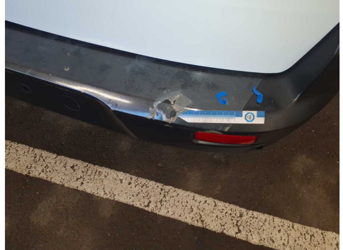
Damage 3: Rear bumper: Rear bumper (unpainted) - Broken / torn - Replace
