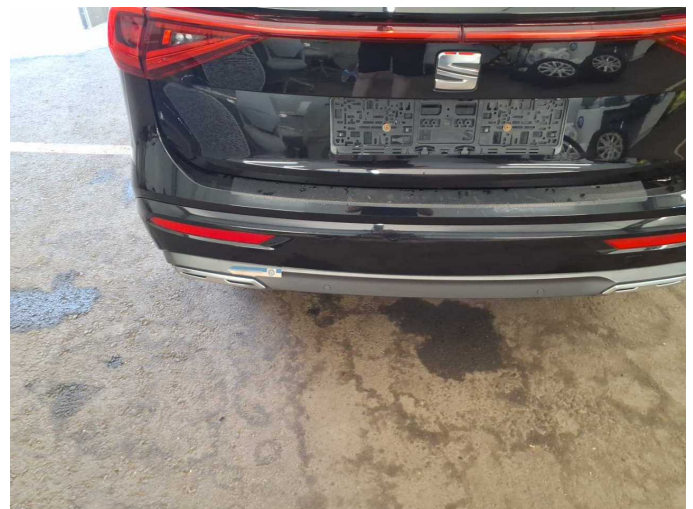
Damage 2: Rear bumper: Spoiler - Scratch(es) - Replace
