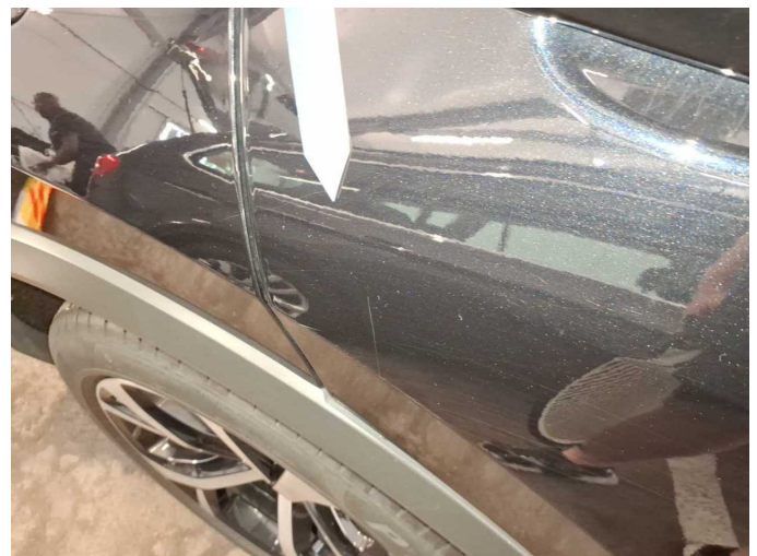
Damage 4: Door - rear right side: Door - Dent / paintcoat damage - Repair and paint
