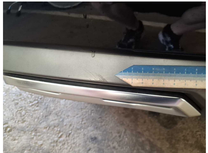
Damage 2: Rear bumper: Spoiler - Scratch(es) - Replace
