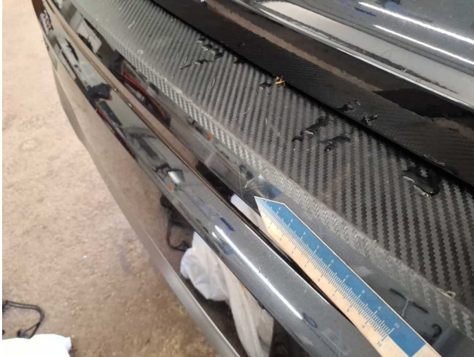
Damage 3: Rear bumper: Rear bumper - Scratch(es) - Paint
