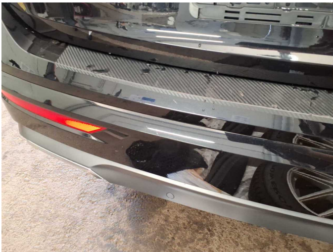
Damage 3: Rear bumper: Rear bumper - Scratch(es) - Paint
