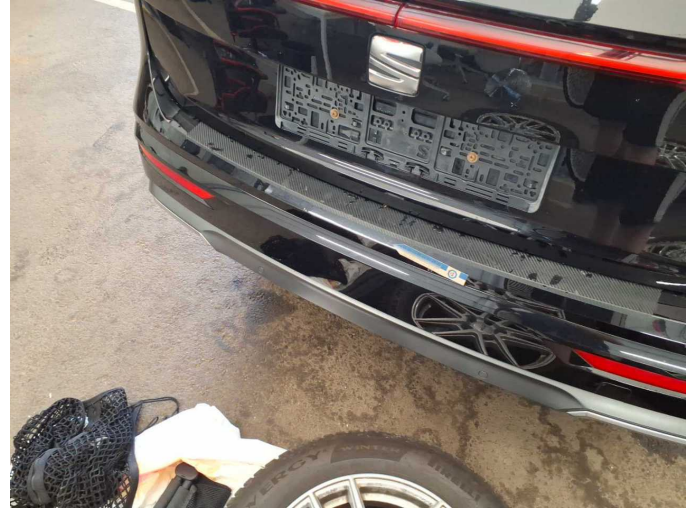
Damage 3: Rear bumper: Rear bumper - Scratch(es) - Paint
