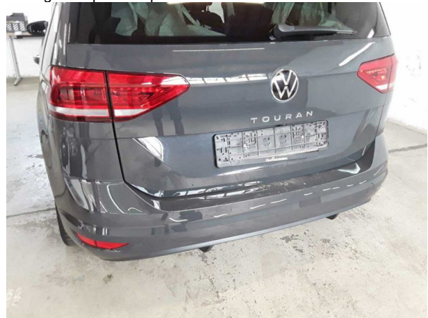
Damage #11: Rear bumper: Rear bumper - Deformed - Replace
