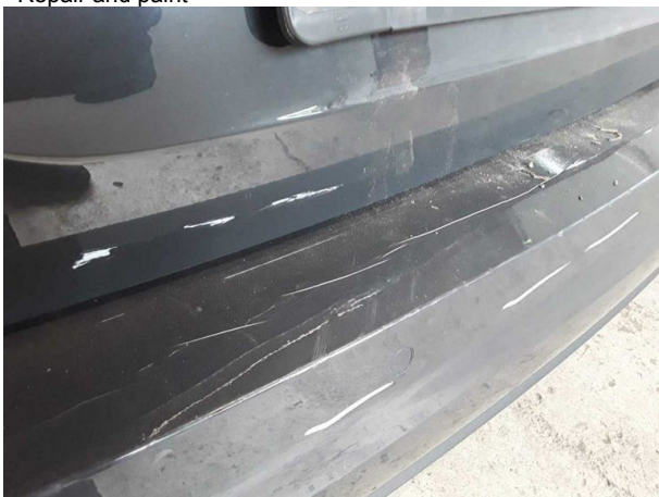
Damage #11: Rear bumper: Rear bumper - Deformed - Replace
