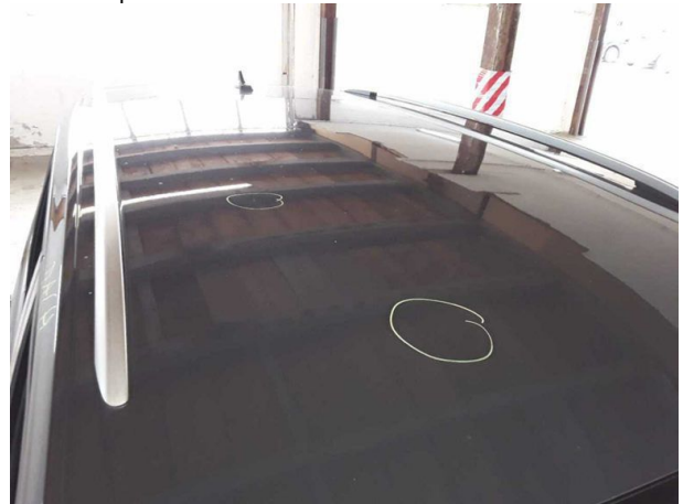
Damage #7: Roof: Roof - dent(s) - Smooth repair work
