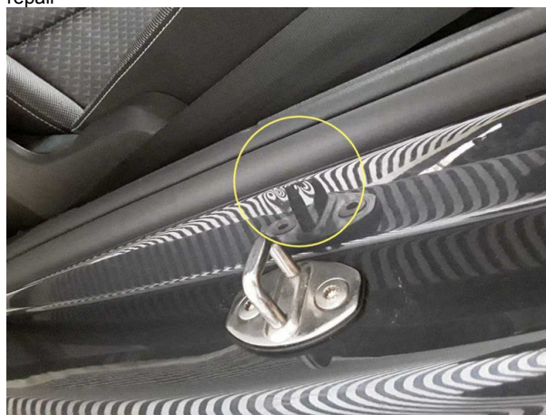
Damage #5: Side panel - rear left side: Sill - dent(s) - Smooth repair work
