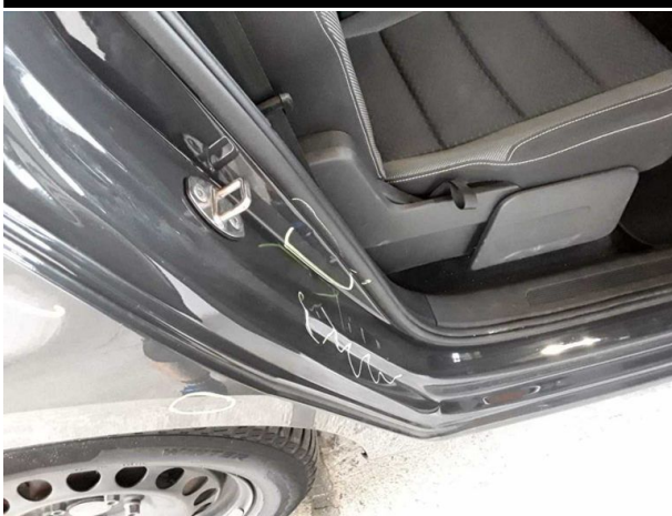
Damage #8: Side panel - rear right side: Sill - Dent / paintcoat damage - Repair and paint
