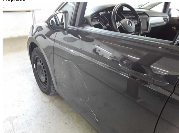
Damage #12: Door - front left side: Door - Deformed - Replace
