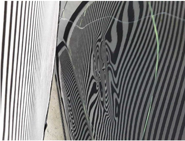
Damage #12: Door - front left side: Door - Deformed - Replace
