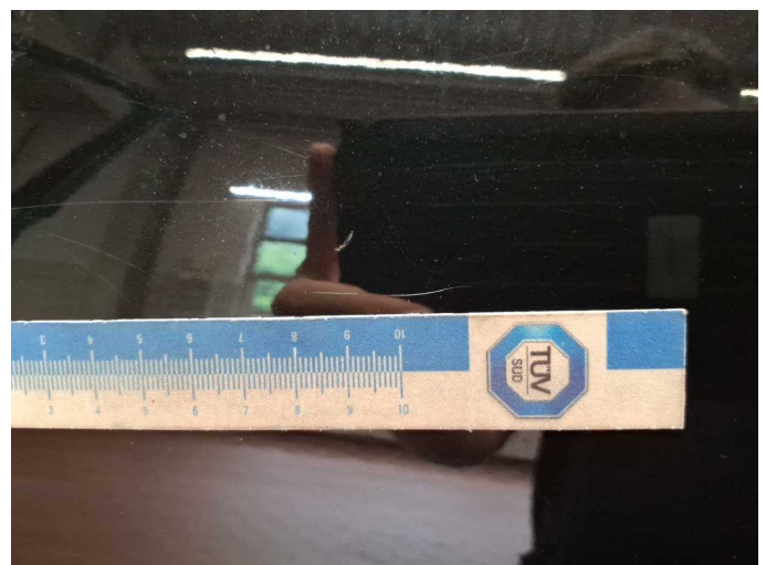
Wear and tear 1: Door - rear left side: Door - Scratch(es) - No deduction
