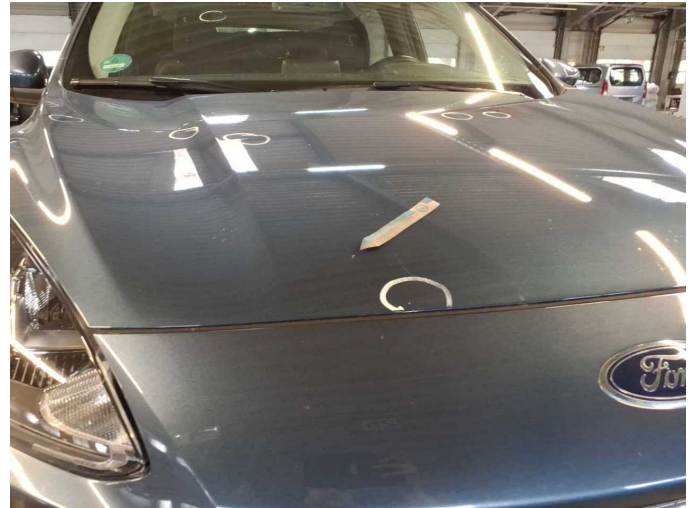
Damage 14: Bonnet: Bonnet (Steinschlag) - Corrosion - Paint
