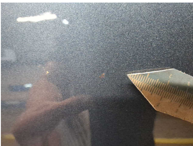
Damage 16: Door - front right side: Door - Dent / paintcoat damage - Repair and paint
