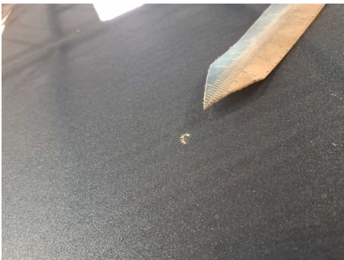
Damage 14: Bonnet: Bonnet (Steinschlag) - Corrosion - Paint
