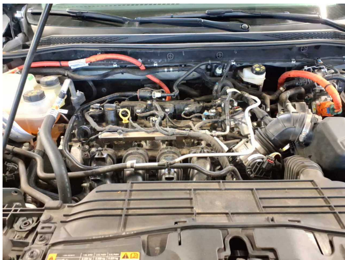
Missing part 1: Engine: Engine cover - Missing - Replace
