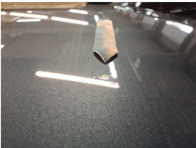
Damage 14: Bonnet: Bonnet (Steinschlag) - Corrosion - Paint
