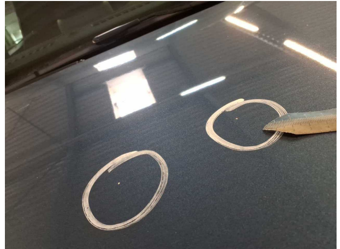
Damage 14: Bonnet: Bonnet (Steinschlag) - Corrosion - Paint
