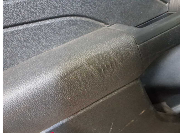
Damage 7: Trim / covers: Door trim - rear left side - Deformed - Replace
