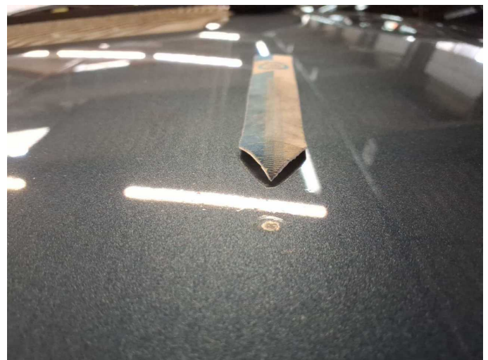
Damage 14: Bonnet: Bonnet (Steinschlag) - Corrosion - Paint
