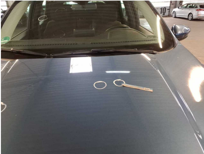
Damage 14: Bonnet: Bonnet (Steinschlag) - Corrosion - Paint
