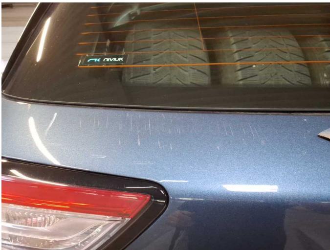
Damage 12: Boot lid / rear door: Boot lid - Dent / paintcoat damage - Repair and paint
