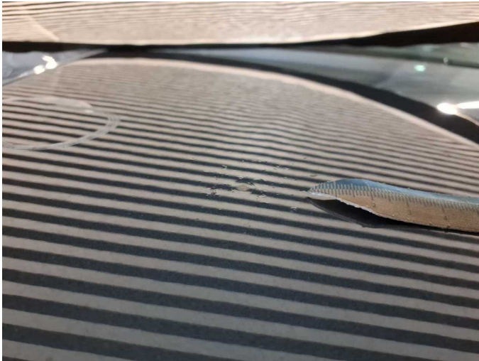
Damage 14: Bonnet: Bonnet (Steinschlag) - Corrosion - Paint
