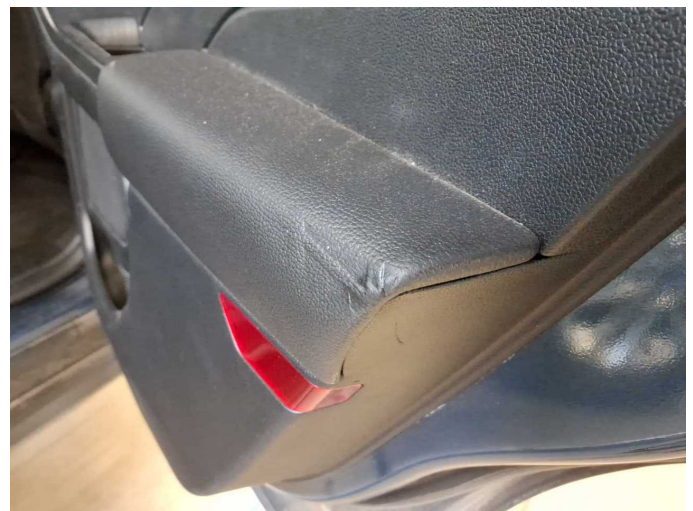
Damage 8: Trim / covers: Door trim - rear right side - Deformed - Replace
