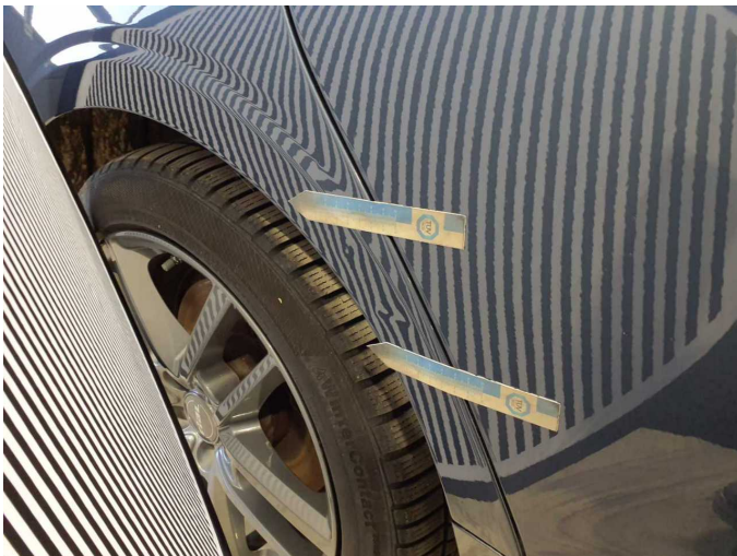
Damage 8: Side panel - rear right side: Side panel - Deformed - Paint
