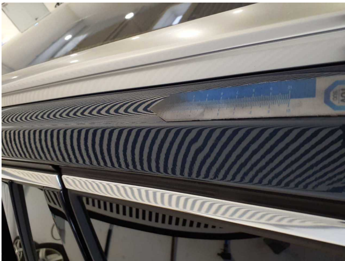
Wear and tear 7: Roof: Roof rail - left side - dent(s) - No deduction
