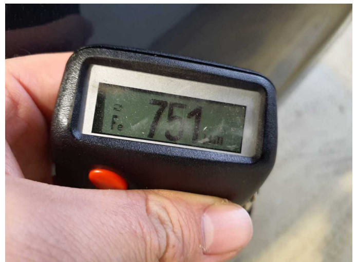
Repainting 1: Roof rail - left side, Side panel - rear left side
