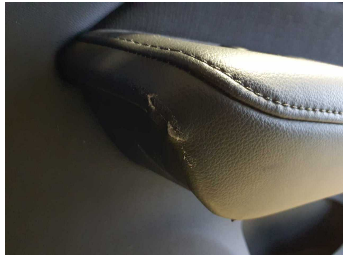
Damage 5: Trim / covers: Door trim - rear right side - Broken / torn - Loss in value
