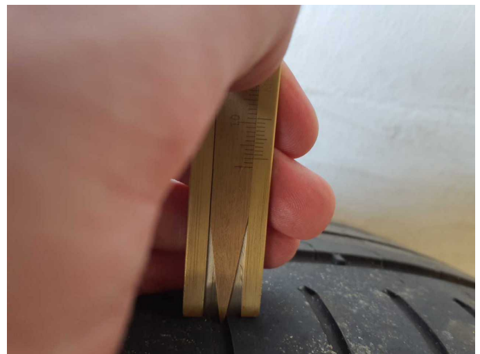
Damage 12: 2nd wheel set: 2 tyres - Worn - Replace
