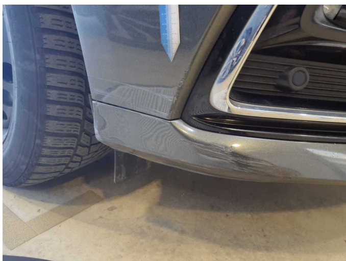
Damage 17: Front bumper: Front bumper (Inklusive anbauteile) - Dent / paintcoat damage - Repair and paint
