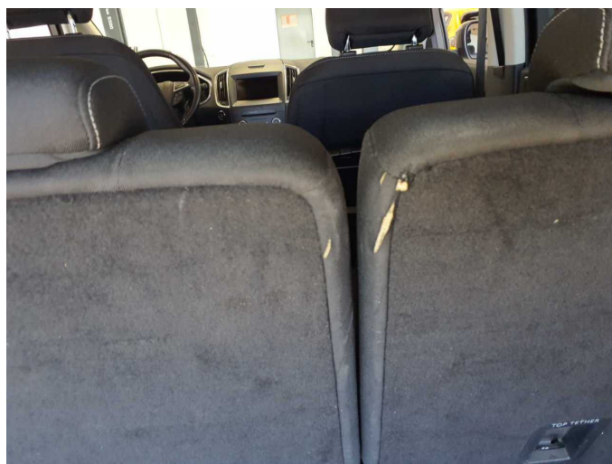
Damage 7: Seat - rear: Upholstery - Broken / torn - Smart repair
