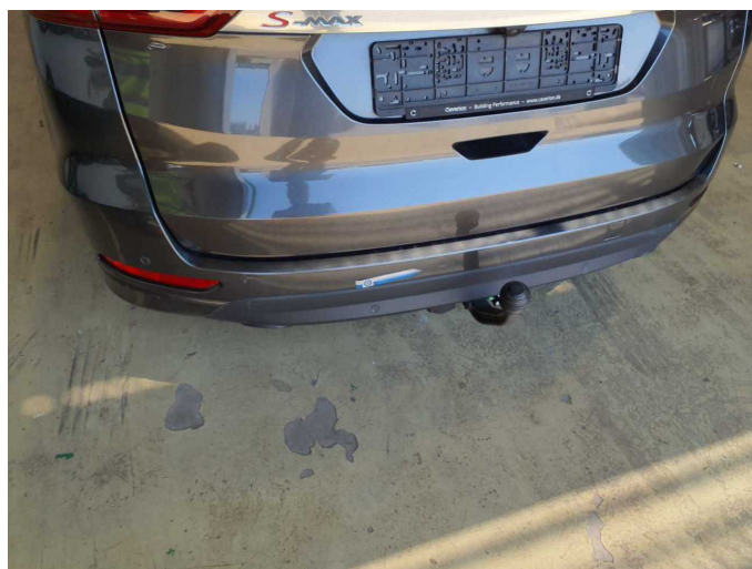
Damage 16: Rear bumper: Rear bumper (Inklusive anbauteile) - Dent / paintcoat damage - Repair and paint
