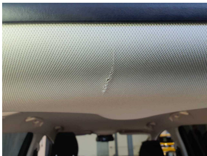
Damage 6: Trim / covers: Roof lining - Scratch(es) - Loss in value
