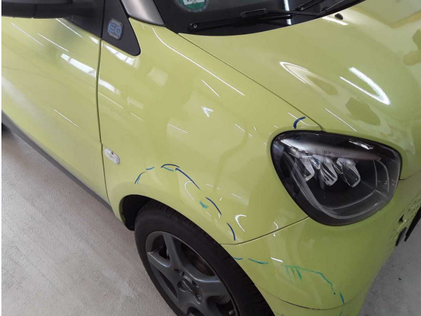
Damage #3: Mudguard - right side: Mudguard - right side - Scratched - Repair and paint
