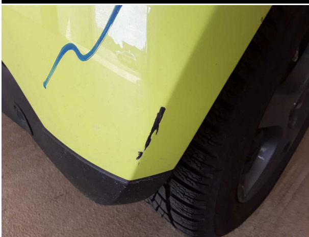
Damage #5: Rear bumper: Rear bumper - Scratched - Repair and paint
