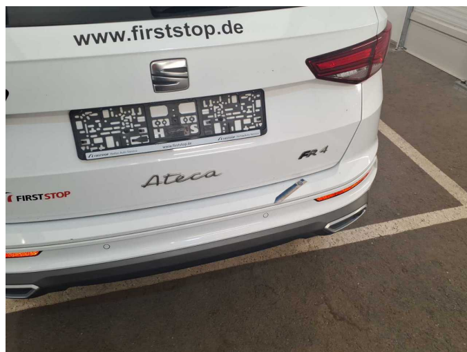
Damage 4: Rear bumper: Rear bumper - Scratch(es) - Paint
