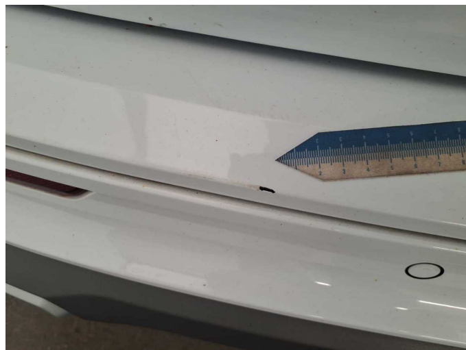
Damage 4: Rear bumper: Rear bumper - Scratch(es) - Paint
