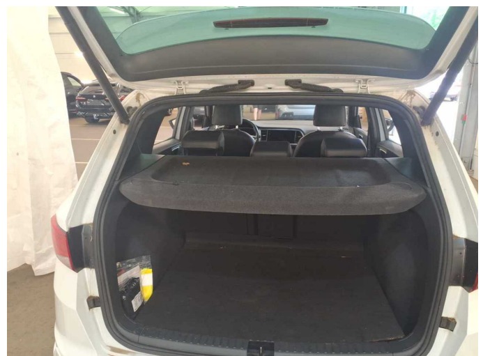
Damage 1: Interior: Rear shelf - Broken / torn - Replace
