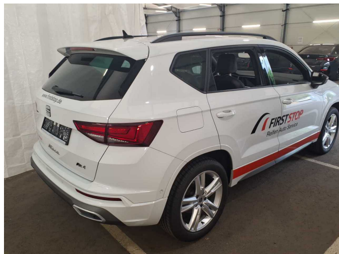
Damage 2: Body: Body - Glued / labelled - De-glue / neutralise
