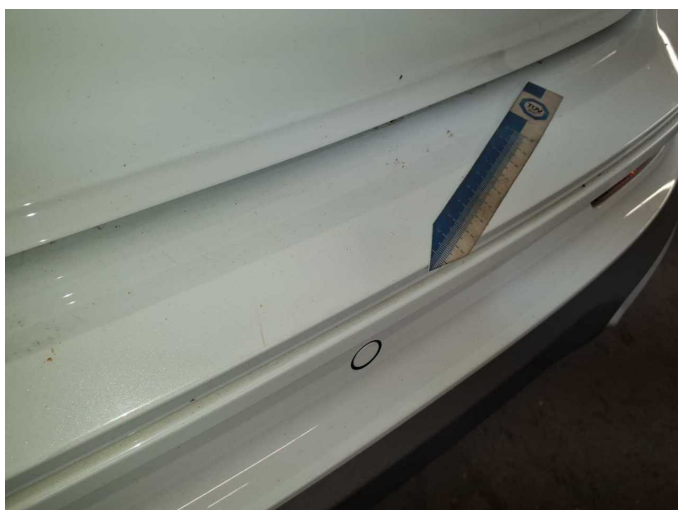
Damage 4: Rear bumper: Rear bumper - Scratch(es) - Paint
