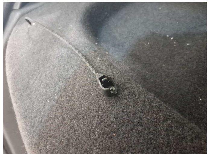
Damage 1: Interior: Rear shelf - Broken / torn - Replace
