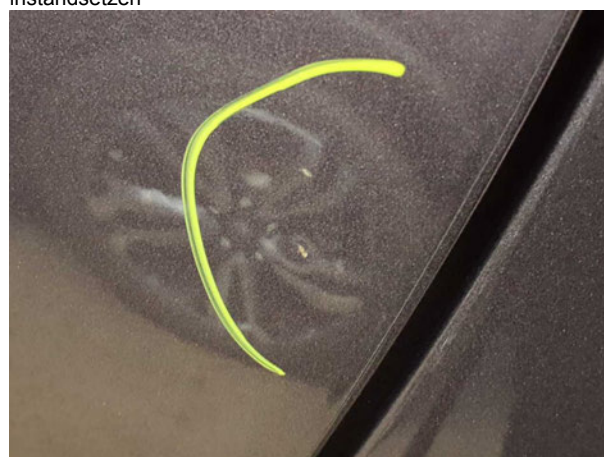
Beschädigung #10: Tür hinten links: Türkante - Delle / Lackschaden - Smart Repair
