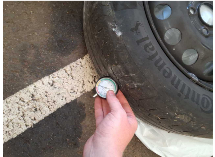
Damage 4: 2nd wheel set: 1 tyre - Does not meet the leasing specifications - Replace
