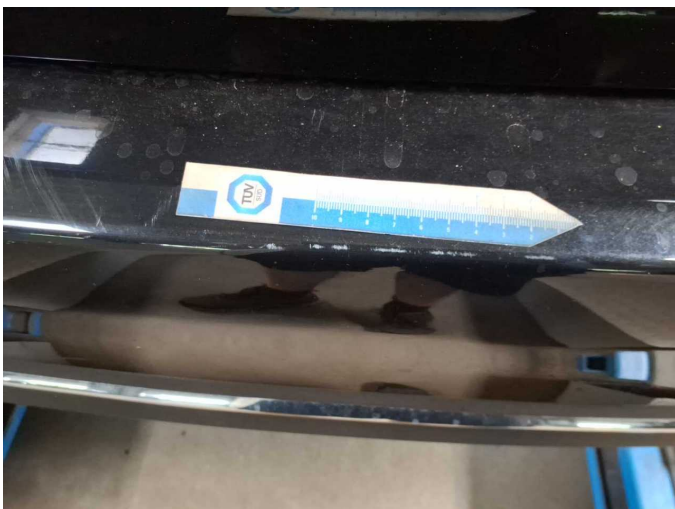
Damage 3: Rear bumper: Rear bumper - Scratched - Paint
