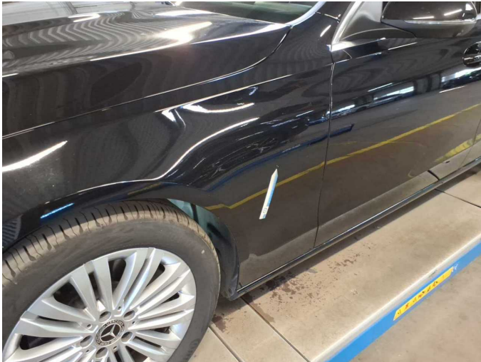
Damage 2: Mudguard - left side: Mudguard - left side - Dent / paintcoat damage - Repair and paint
