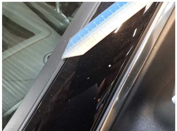
Damage 1: Body: A-pillar - left side - Stone chips - Smart repair
