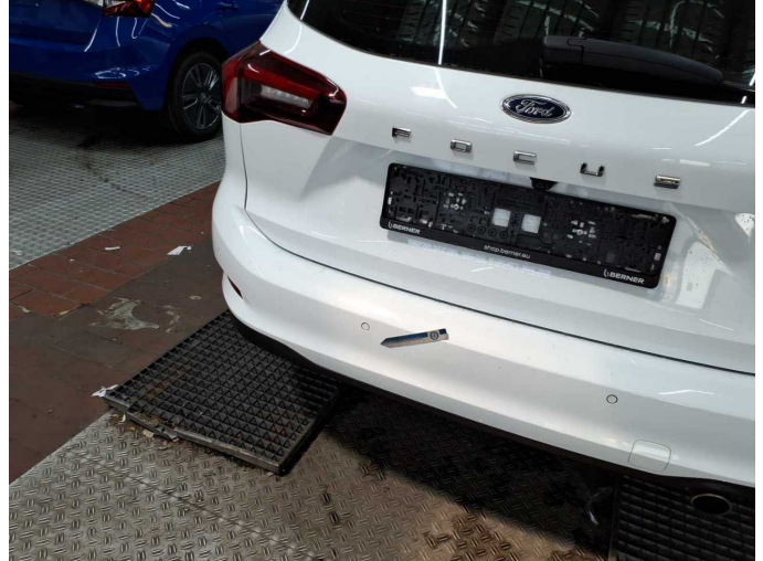
Damage 1: Rear bumper: Rear bumper - Abrasion - Smart repair
