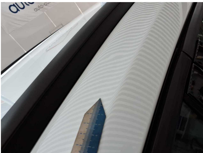
Wear and tear 4: Roof: Roof rail - left side - dent(s) - No deduction
