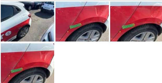
Door RL, Bad repair, Paint
