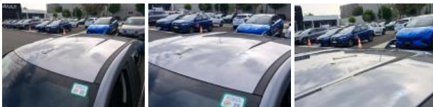
Roof, Hail damage, Repair and paint (complete)
