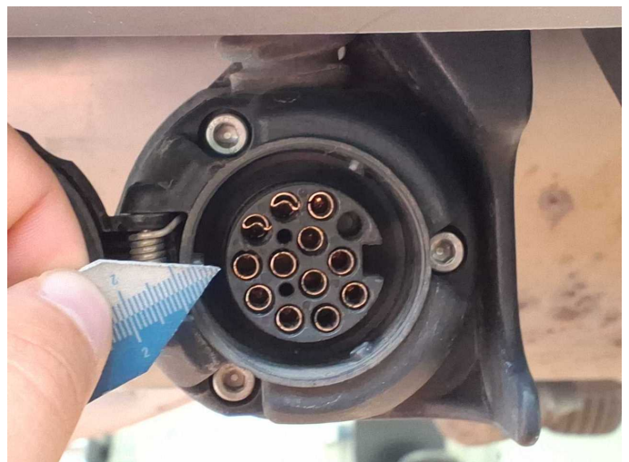
Damage 1: Trailer hitch: Electrical connection socket (Pins Verformt) - Deformed - Replace
