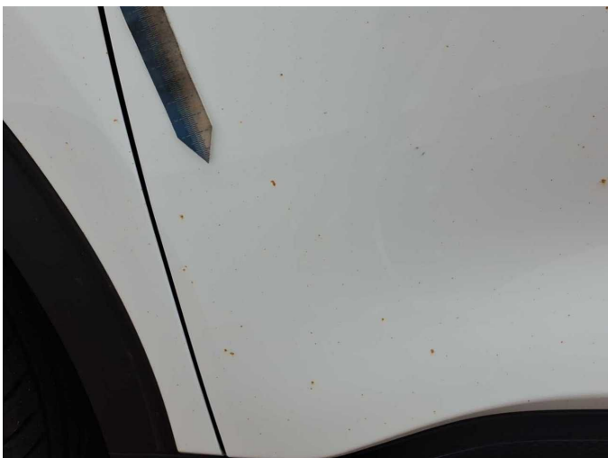
Damage 6: Body: Body (Flugrost) - Corrosion - Conditioning
