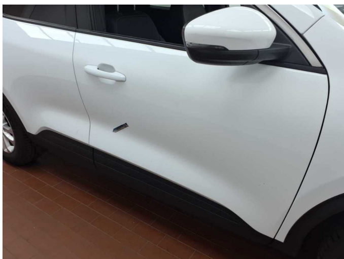
Damage 6: Body: Body (Flugrost) - Corrosion - Conditioning
