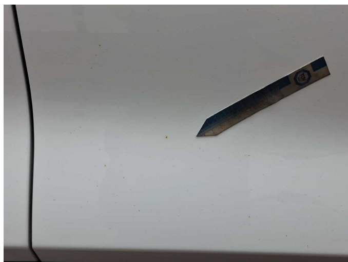
Damage 6: Body: Body (Flugrost) - Corrosion - Conditioning
