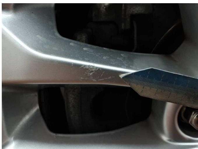
Damage 10: Wheel / tyres: Alloy rim - front left side - Scratched - Loss in value
