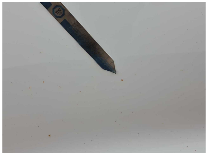
Damage 6: Body: Body (Flugrost) - Corrosion - Conditioning
