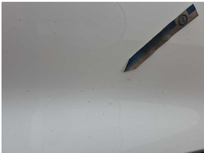
Damage 6: Body: Body (Flugrost) - Corrosion - Conditioning
