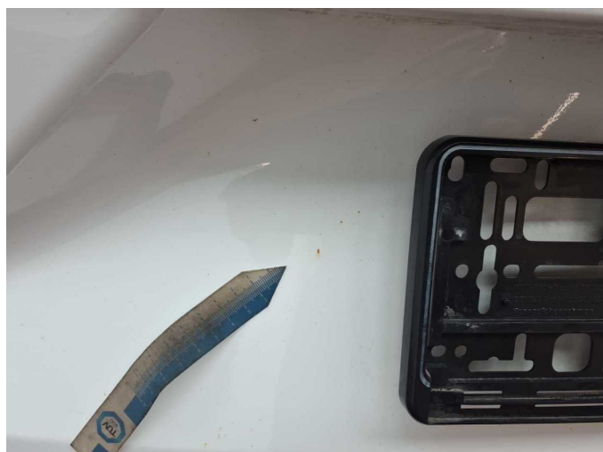
Damage 6: Body: Body (Flugrost) - Corrosion - Conditioning
