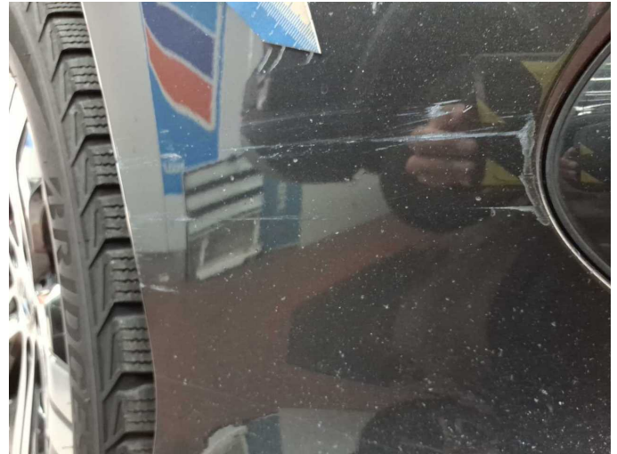
Damage 2: Front bumper: Front bumper (inkl. Zierblende rechts erneuern) - Scratched - Repair and paint
