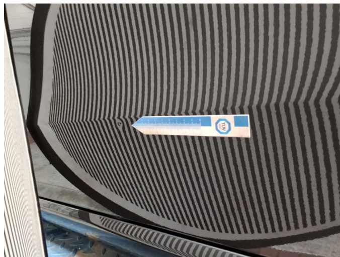
Damage 1: Door - rear left side: Door - dent(s) - Smart repair
