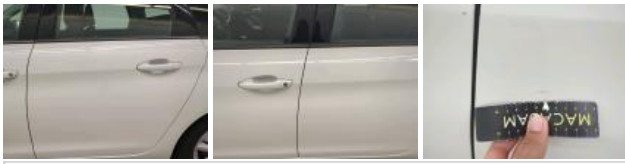
Wing RL, Scratch(es), Repair and paint (complete)
