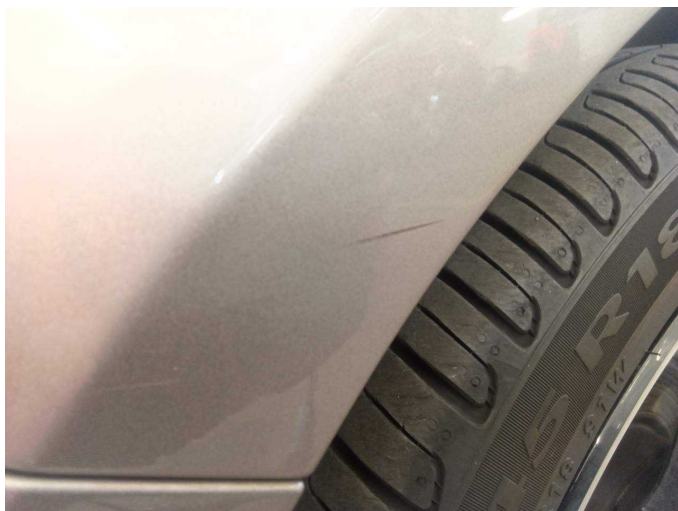
Wear and tear 2: Mudguard - left side: Mudguard - left side - Scratch(es) - No deduction
