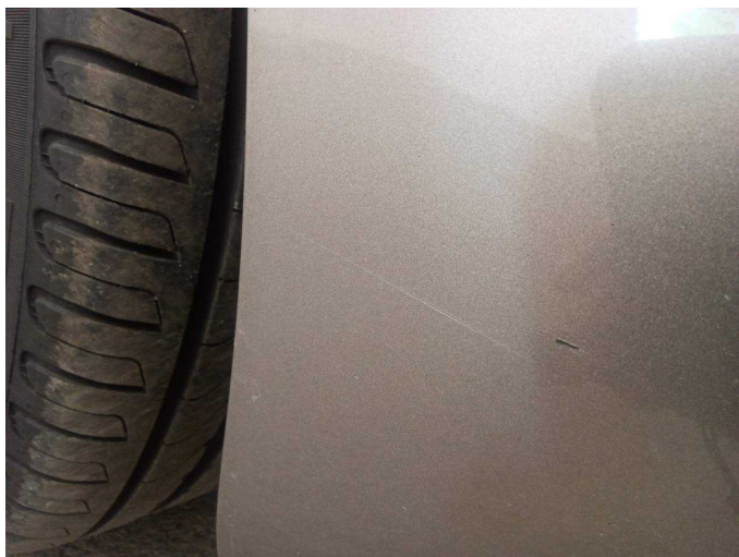
Damage 12: Front bumper: Front bumper - Scratch(es) - Paint
