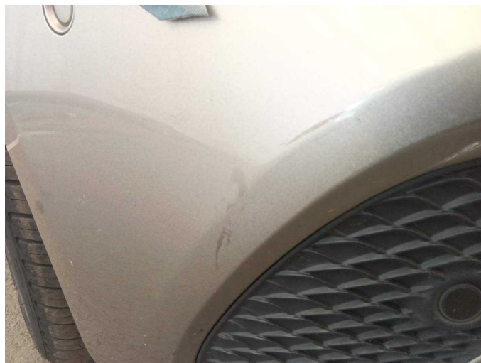
Damage 12: Front bumper: Front bumper - Scratch(es) - Paint
