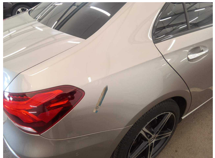
Damage 11: Side panel - rear right side: Side panel - Scratch(es) - Paint
