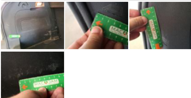
Garnit zone de chargement, Griffe(s), Acceptable
