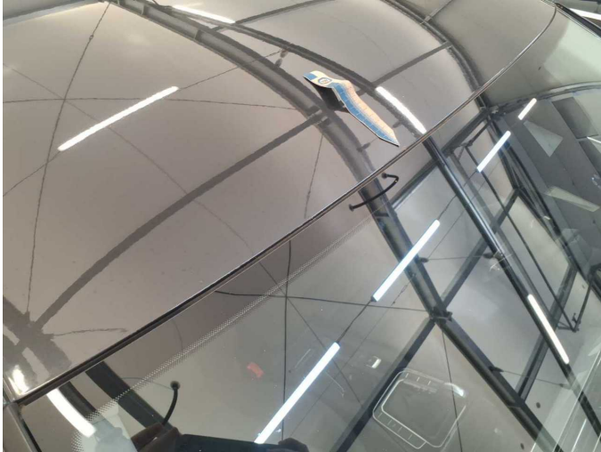
Damage 4: Roof: Roof - Stone chips - Repair and paint
