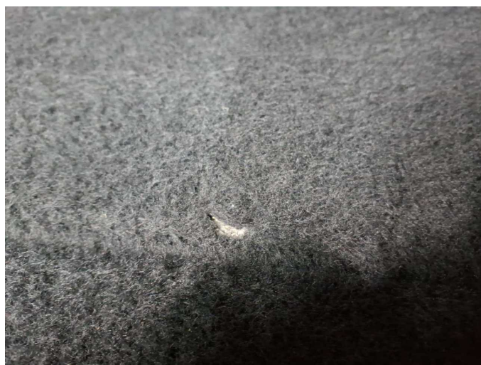
Damage 5: Interior: Cargo area floor - Holes - Replace
