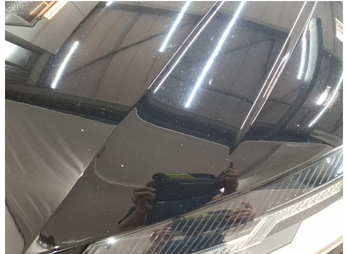
Damage 8: Bonnet: Bonnet - Stone chips - Paint
