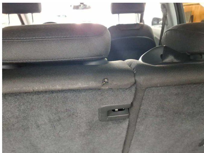
Damage 4: Seat - rear: Upholstery - Holes - Loss in value
