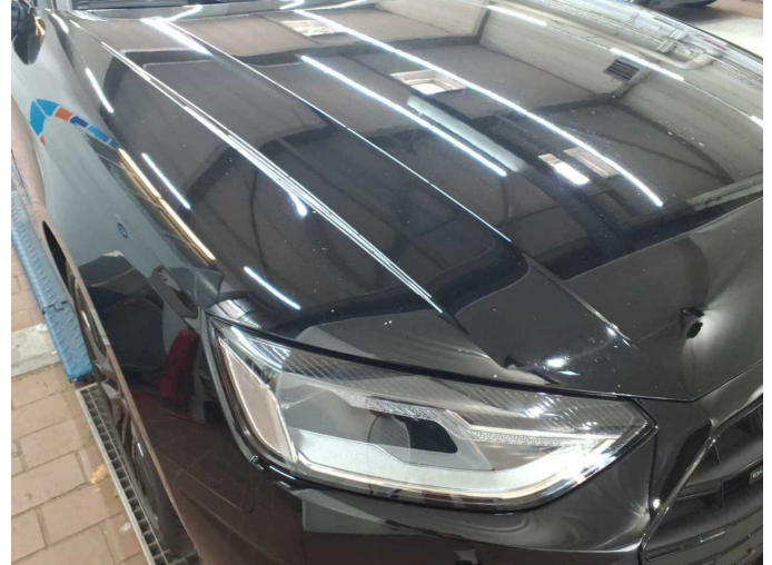
Damage 8: Bonnet: Bonnet - Stone chips - Paint
