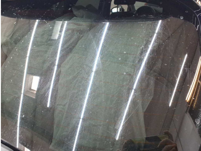
Damage 7: Vehicle glazing: Rear window - Scratch(es) - Replace
