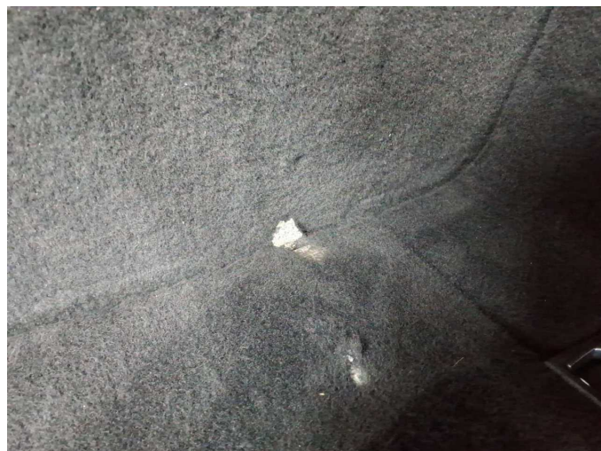
Damage 5: Interior: Cargo area floor - Holes - Replace
