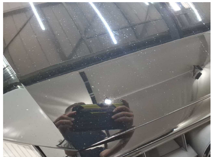
Damage 8: Bonnet: Bonnet - Stone chips - Paint
