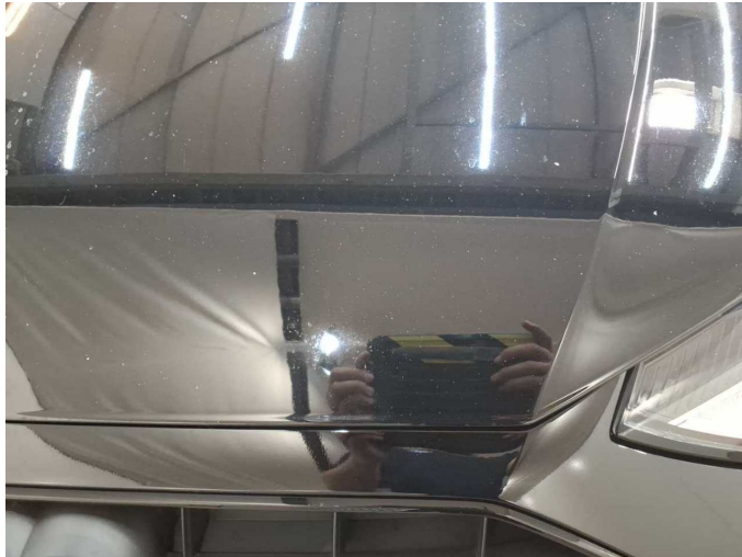
Damage 8: Bonnet: Bonnet - Stone chips - Paint
