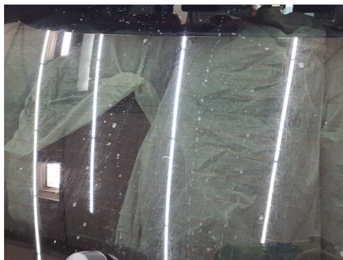
Damage 7: Vehicle glazing: Rear window - Scratch(es) - Replace
