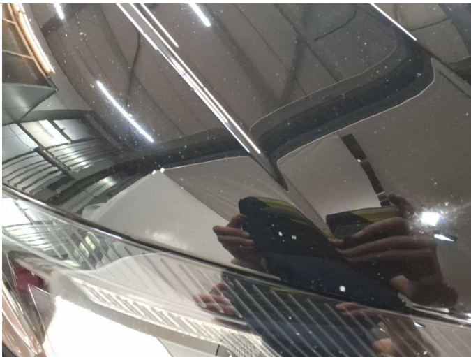
Damage 8: Bonnet: Bonnet - Stone chips - Paint
