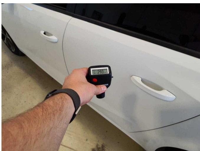
Repainting 2: Door - rear left side
