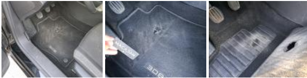
Floor covering FL, Burned, Smart repair
