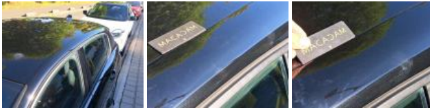
Door RL, Scratch(es), Repair and paint (complete)
