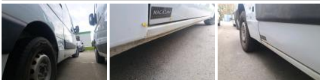
Outer sill R, Bad repair, Repair and paint (complete)
