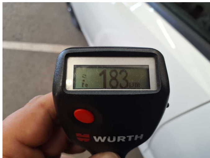
Repainting 1: Door - front left side
