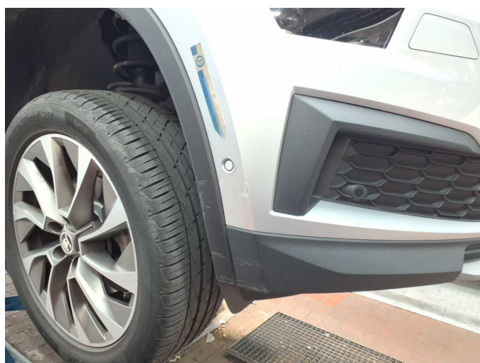
Damage 6: Front bumper: Front bumper (inkl. Radlauf re.) - Scratch(es) - Paint
