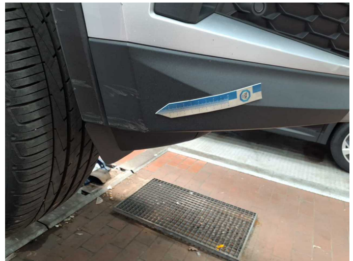
Damage 2: Front bumper: Spoiler - Scratch(es) - Smart repair
