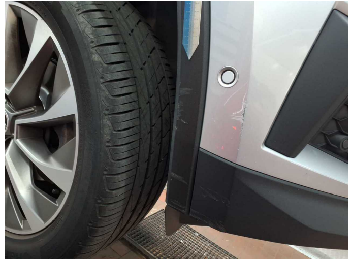
Damage 1: Mudguard - right side: Wheel well extension - Scratch(es) - Smart repair
