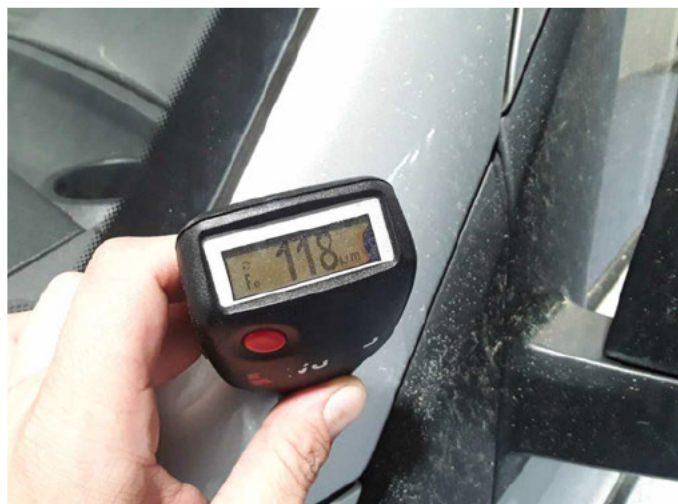
Dachholm links: 118 µm
