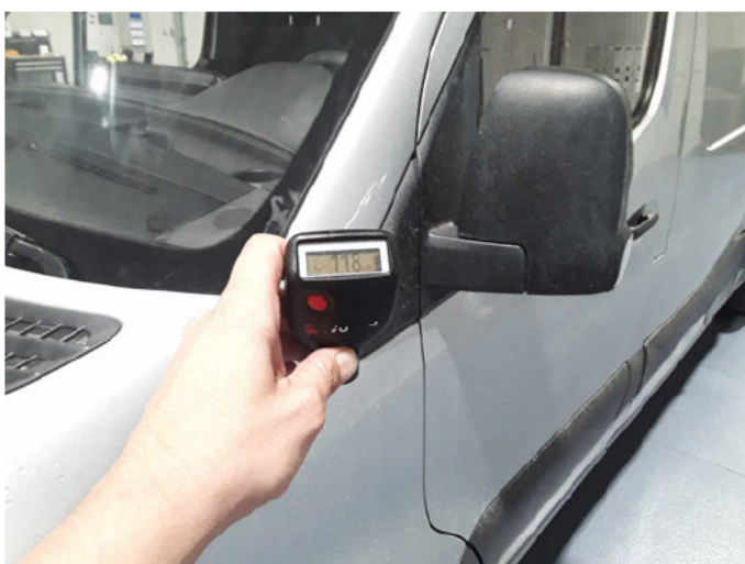
Dachholm links: 118 µm
