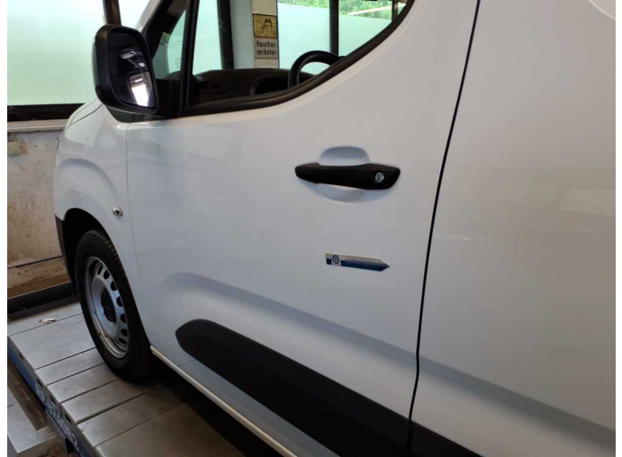
Damage 6: Door - front left side: Door - Deformed - Repair and paint
