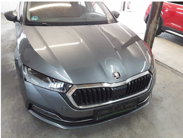
Damage #4: Bonnet: Bonnet - dent(s) - Smooth repair work
