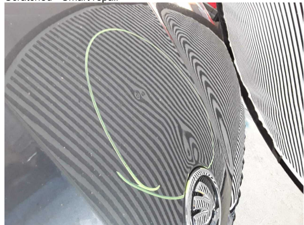
Damage #4: Bonnet: Bonnet - dent(s) - Smooth repair work
