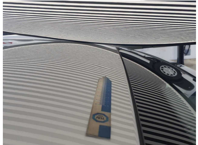
Damage 2: Roof: Roof - dent(s) - Smooth repair work
