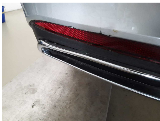
Damage 5: Rear bumper: Rear bumper - Deformed - repair according to calculation
