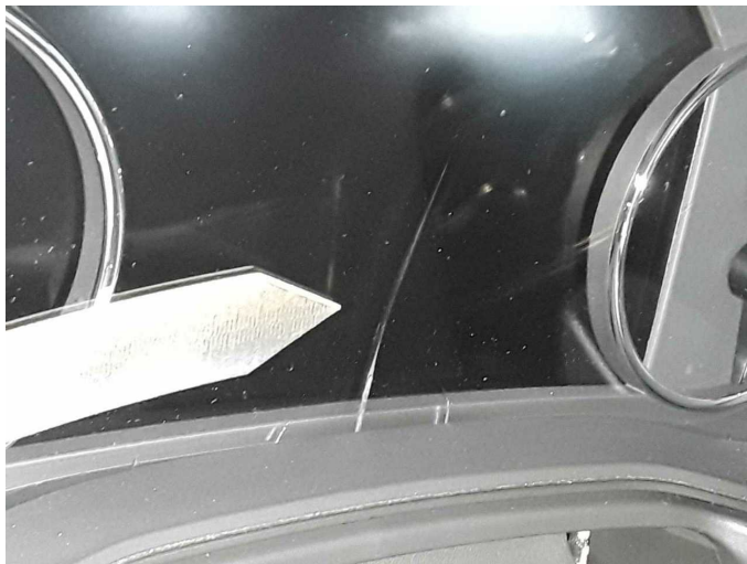
Damage 6: Instrument panel: Instrument cluster - Broken / torn - Replace
