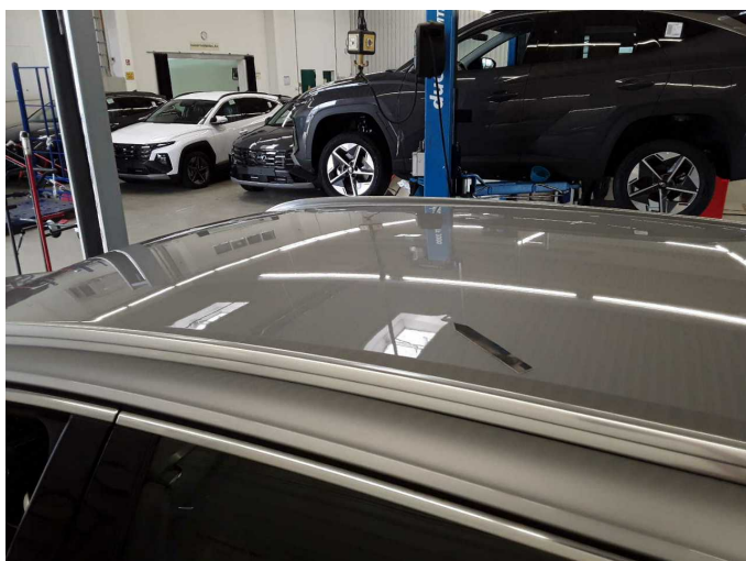
Damage 1: Roof: Roof - dent(s) - Smart repair
