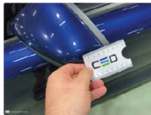
4 - Inner door sill FL - Dent(s) and scratch(es)
