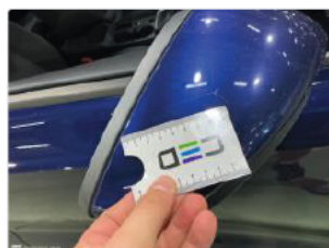
8 - Outside rear-view mirror housing R - Scratch(es)
