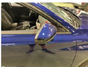
8 - Outside rear-view mirror housing R - Scratch(es)
