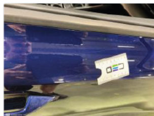
8 - Outside rear-view mirror housing R - Scratch(es)
