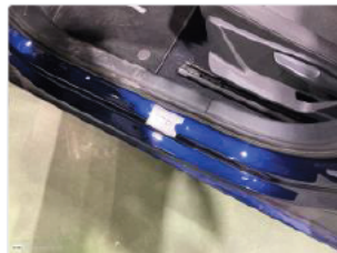
4 - Inner door sill FL - Dent(s) and scratch(es)
