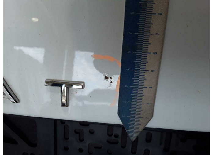
Damage 5: Boot lid / rear door: Boot lid - Corrosion - Repair and paint
