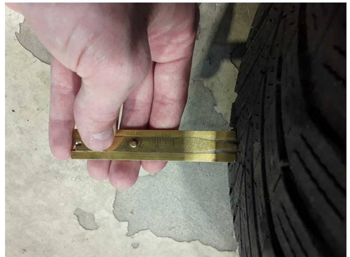
Damage 1: 2nd wheel set: 2 tyres - does not meet manufacturer specifications - No deduction
