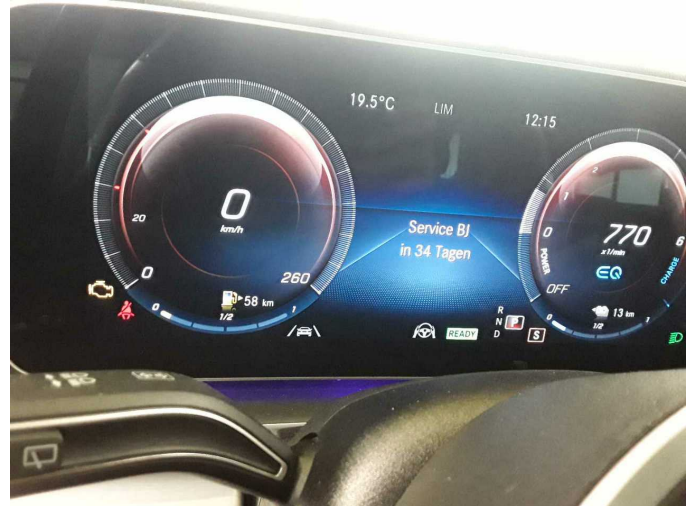
Damage 8: Instrument panel: Indicator light (MKL) - on - Perform diagnosis
