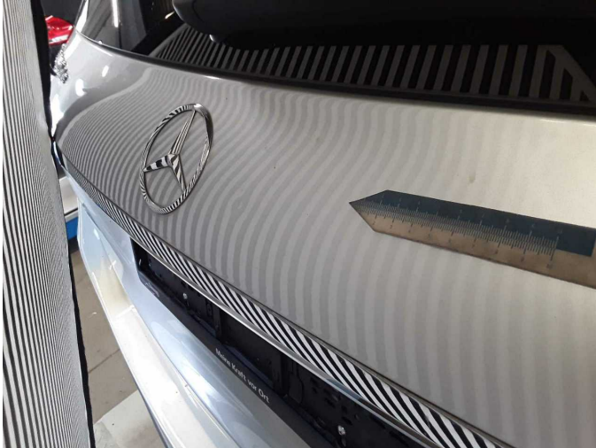
Damage 7: Boot lid / rear door: Boot lid - Dent / paintcoat damage - Smart repair
