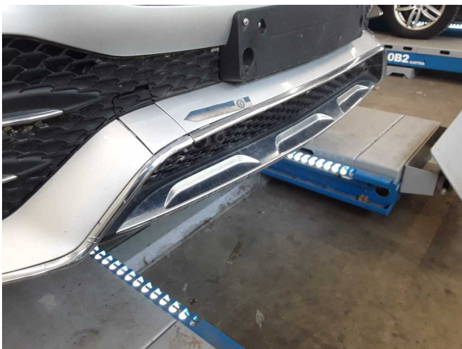
Damage 10: Trim / covers: Brightware / decorative strip (+ lose (Stoßstange vorne)) - Paint defect - Replace
