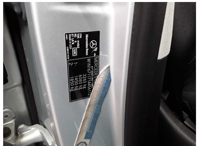
Damage 1: Body: Identification plate - Damaged - Replace
