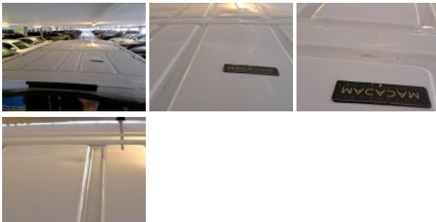
Roof, Dent(s), Repair and paint (complete)
