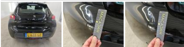
Bumper RM, Crack, Replace
